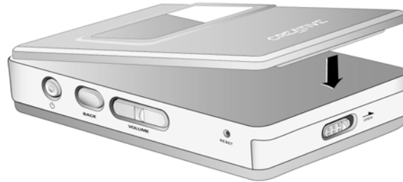
Figure 2-3: Securing the cover.
